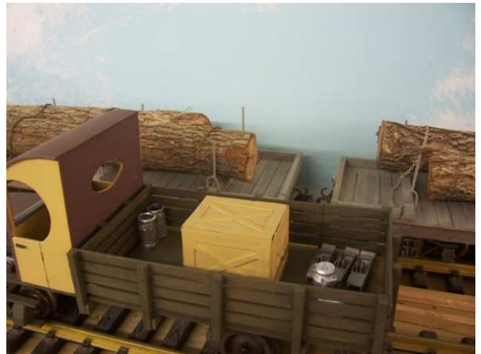
Cab made from 2mm styrene, under-frame and rear tray are 2mm plywood, side gates are split pine.
