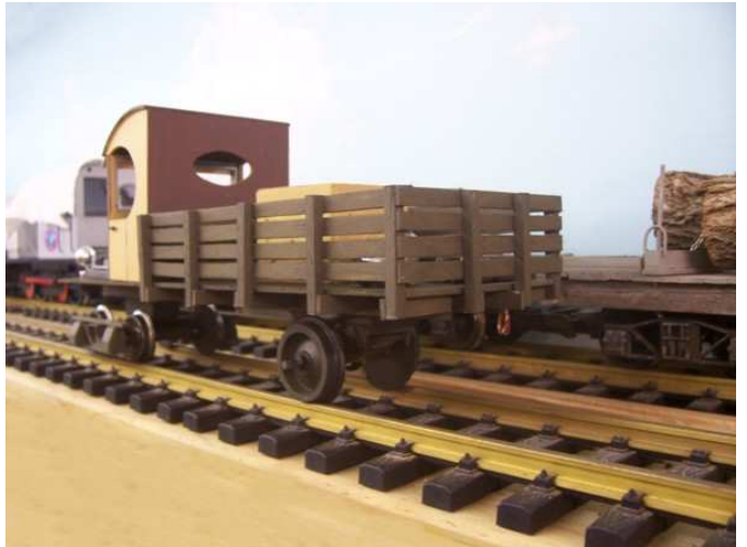
Leading bogie made from Styrene & Brass.
